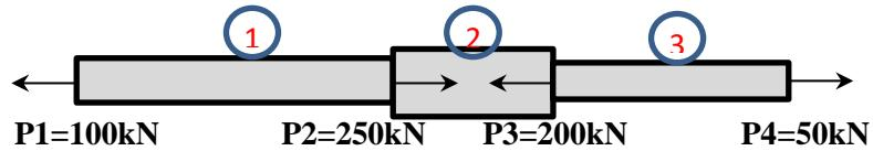
Take the lengths and areas as 2 meter, 1000 mm<sup>2</sup>, 1meter, 2000 mm<sup>2</sup> and 1.5 meter, 1000 mm<sup>2</sup> for sections 1 to 3 respectively, and E=207GPa for all sections.
