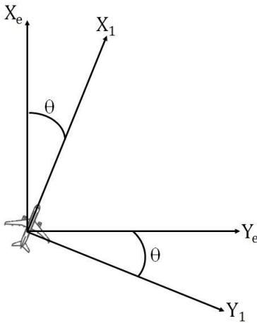
The transformation matrix  $T$  can be derived by expressing the unit vectors of system 1 in terms of the unit vectors of system e. Derive the expression for the transformation matrix.
