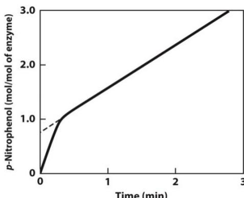
i. Initially, the reaction releases a rapid burst of p-nitrophenol nearly stoichiometric with the amount of enzyme present. The subsequent rate is slower. Provide a plausible explanation for this evidence.
