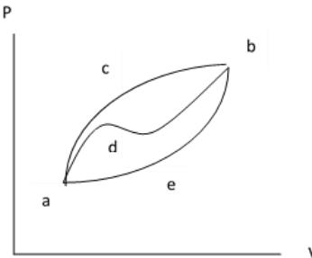
When a system is taken from state a to state b along the path acb, 100 J of heat flows into the system and the system does 40 J of work.
