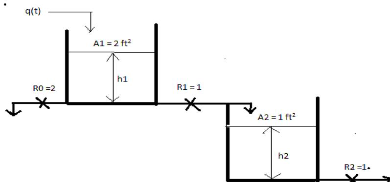
Note:  $A_1 = 2 \text{ ft}^2$ ;  $A_2 = 1 \text{ ft}^2$ ,  $R_0 = 2$ ,  $R_1 = 1$ , and  $R_2 = 1$  for the above diagram.
