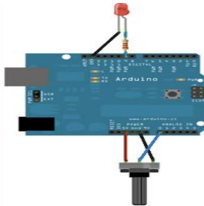
Analyze how digital Read/Write pins behave like analog Write pins considering the following circuit diagram: (LED- 9, Potentiometer – A0). Write the code for the given circuit.
