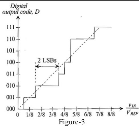
b) Determine the INL for the 3 bit ADC whose transfer curve is shown in Fig-4. Assume that  $V_{REF} = 5$  V. Draw the quantization error,  $Q_e$ , in units of LSBs.
