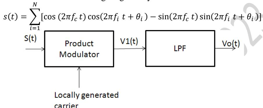
i) Show that the modulation can be completely recovered if the cutoff frequency of the filter  $f_N < f_o < 2f_c$
