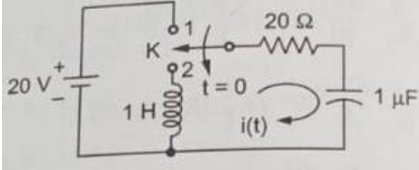
b) The network shown in figure has two independent node pairs of the switch K is opened at  $t=0$ , Calculate the following quantities at  $t=0$  i)V<sub>1</sub> ii)V<sub>2</sub> iii)dV<sub>1</sub>/dt iv)dV<sub>2</sub>/dt
