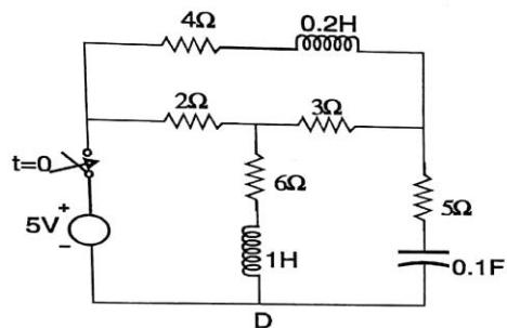
c) For the network shown in figure draw the network graph, select a tree and write a tie-set schedule.
