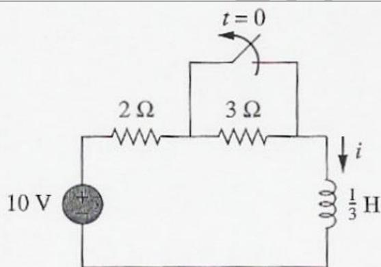
Assume the circuit shown in fig 6.1 has been closed for a long time. Find  $i$  at  $t=0^+$  and  $i$  at  $t=\infty$
