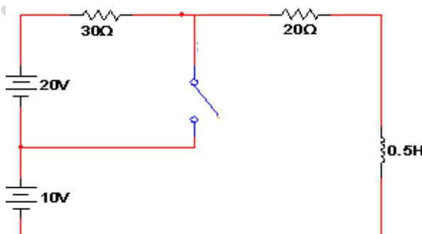
b) In the network steady state is reached with the switch K open. At  $t = 0$ , switch is closed. Determine the values of  $V_a(0^-)$  and  $V_a(0^+)$
