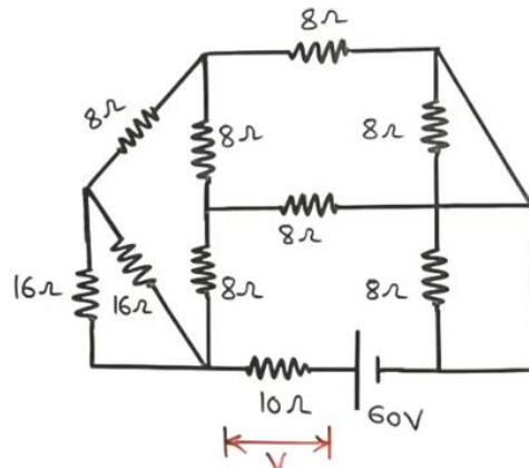
b) Reduce the network shown in fig. into a single current source in parallel with one of the elements. 08
