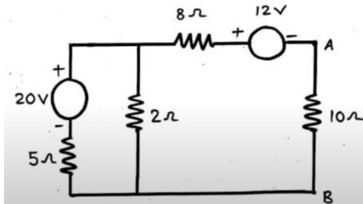
b) For the circuit shown below find the load resistance  $R_L$  to have maximum power dissipated. Also find that maximum power.
