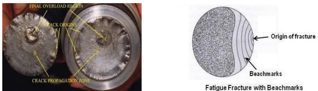
Fig.3 Mechanism of fatigue failure
