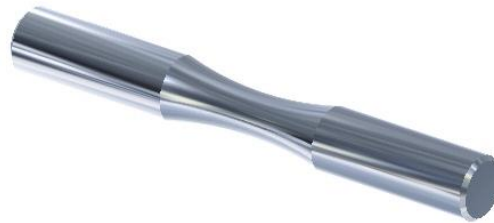
Fig.5. Rotating Bending test machine and Test specimen for
