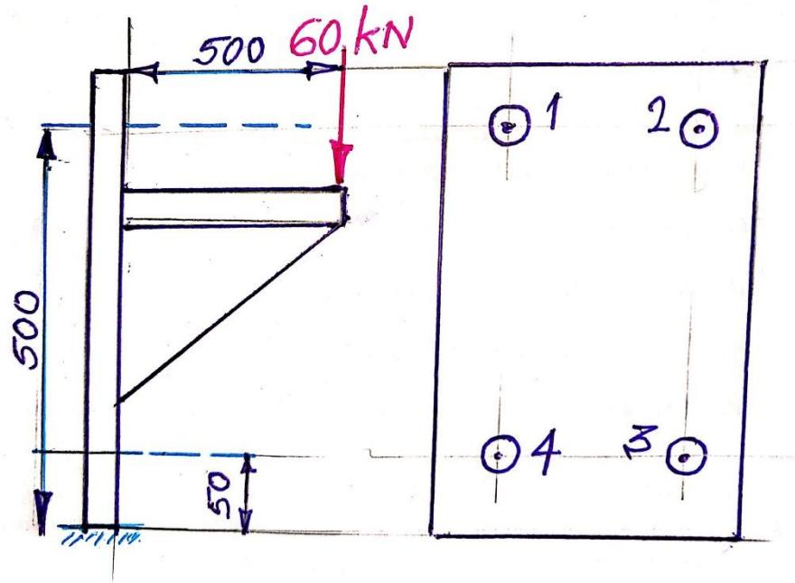
Primary load is shear load
