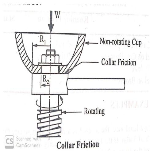
**Collar friction:** Torque required to overcome collar friction
