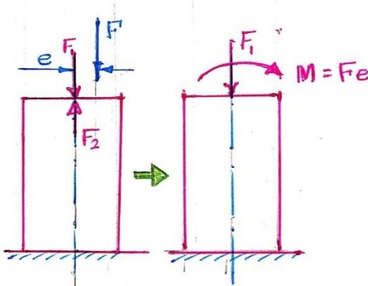
Effect of Direct load and Moment need to be considered in designing eccentrically loaded bolted joints
