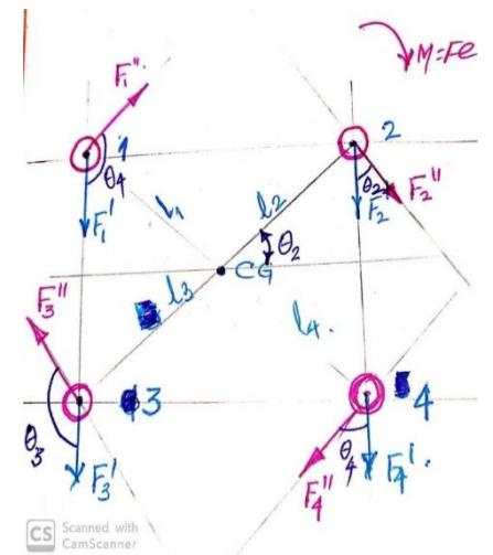
2. Draw the loading diagram showing the primary and secondary forces as shown above
