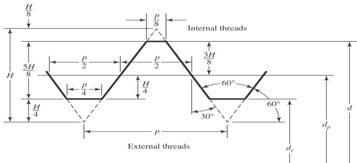
**Coarse and fine threads:** Coarse threads are used in applications free from vibrations: Fine threads are used under dynamic loads.
