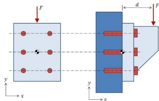
**Load axis parallel to the bolt axis**
