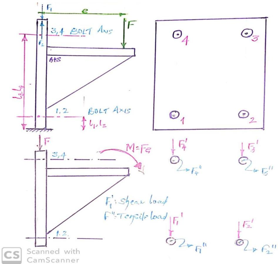
Load axis perpendicular to the bolt axis. Applied load tends to turn the bracket about the titling edge which is shown by hatched line.
