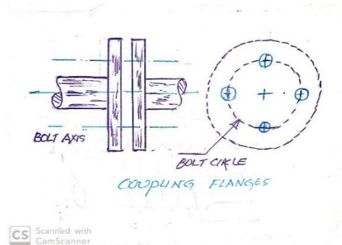
Shear force that can be transmitted by each bolt
