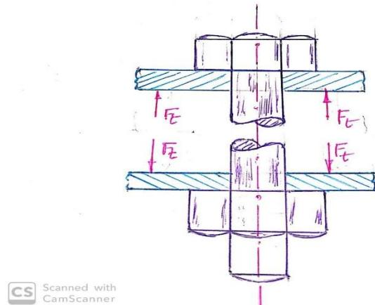
**Torsional stress due to friction between threads:** When torque is applied on the screw rod either to tighten the nut or to drive in a screw torsional shear stresses are induced in the body of the screw. It is given by:
