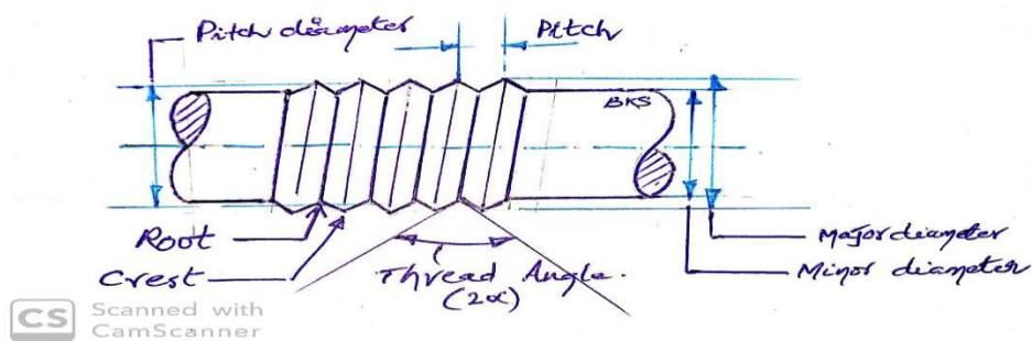
**Major diameter:** Nominal diameter: Diameter of an imaginary cylinder that bounds the crests of an external thread or roots of an internal thread.
