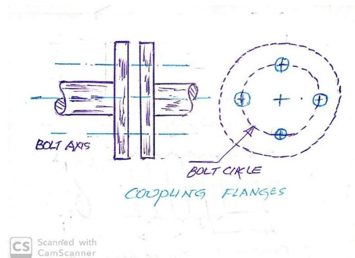
Bolts are subjected to shear load. Shank of the bolts are sheared off.
