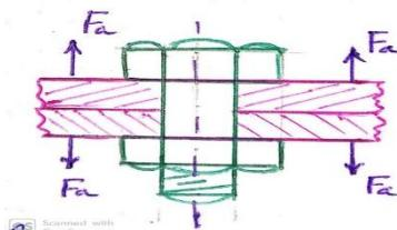
b) **Joints for pressure vessels and cylinder heads:** Functional requirement is to hold the parts together and also making the joint leak proof. Gaskets are used as shown Eg; Cylinder Head. Bolts are subjected to direct tensile stresses due to pressure of the fluid inside the cylinder. The gas forces tend to push the cylinder head outwards which is resisted by the bolts.
